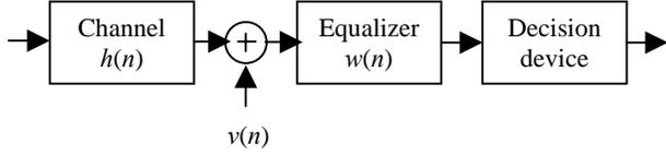
**Fig. 1** Blind equalizer in a digital communication system.
