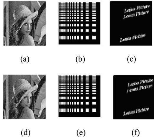
Fig. 7. Robustness of FICA demixing with respect to the JPEG image data compression. (a)-(c): The compressed original images. (d)-(f): The images demixed from compressed mixtures of originals.
