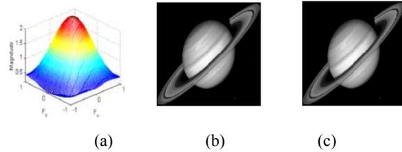
Fig. 1. (a) The frequency response of the specified filter, (b) The original image of Saturn, (c) The watermarked image using 2-D filter.
