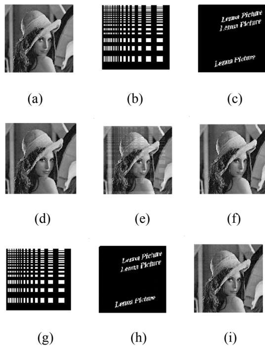
Fig. 4 The watermark extraction results by using the text image as the watermark: (a) The original Lenna image, (b) The key image, (c) The text watermark, (d) The watermarked image, (e) and (f) The generated mixture images, (g) The extracted key, (h) The extracted watermark, (i) The extracted Lenna image.
