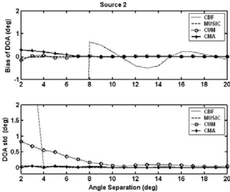
Fig. 3. Performance of DOA estimation for the second source at varying angular separations.
