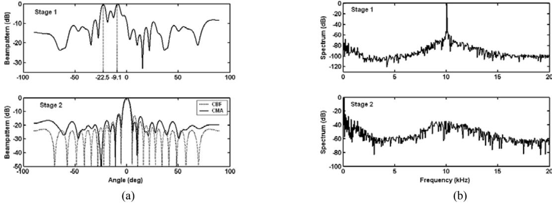
Fig. 7. 16-sensors ULA receive two coherent signals from directions  $(-22.5^\circ, -9.1^\circ)$ . (a) Beampattern of each CM array stage, and (b) Spectra of CM array outputs.
