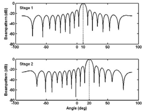
Fig. 2. Beampatterns of two stage CM array. Directions of two independent signals are  $10^\circ$  and  $20^\circ$ , the signal input SNR=[10dB, 5dB].
