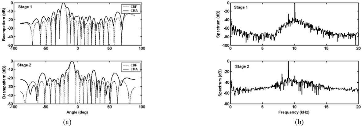
Fig. 6. 16-sensors ULA receive two independent signals from directions  $(-22.5^\circ, -9.1^\circ)$ . (a) Beampattern of each stage CM array, and (b) Spectra of CM array outputs.
