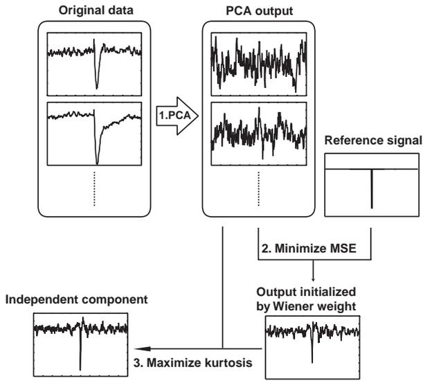
**Fig. 1.** Conceptual three stage for extraction desired ICs.
