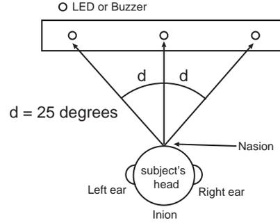
**Fig. 3.** Placement of LEDs.
