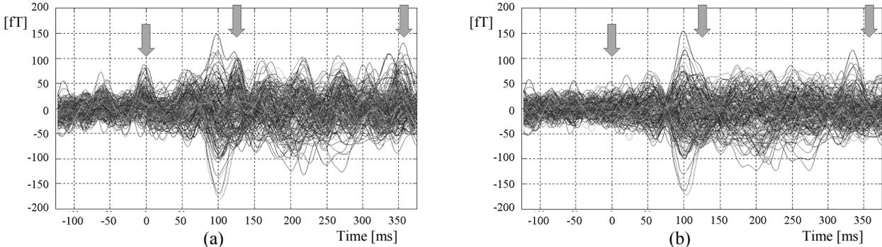
Figure 5 Superimposed traces of auditory evoked magnetic field obtained by averaging 30 epochs. (a): without and (b): with the proposed ICA noise reduction.
