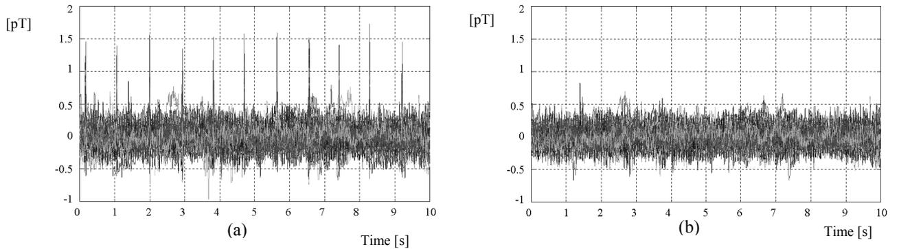
Figure 3 (a) The superimposed traces of non-averaged magnetic fields measured with repeated stimulus of tone bursts (see text). (b) The same data noise reduction by ICA. The cardiac activity has been removed.
