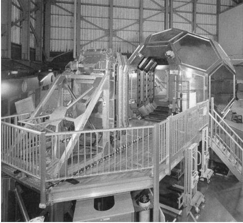
Figure.1 A magnetically shielded room at Tokyo Denki University.
