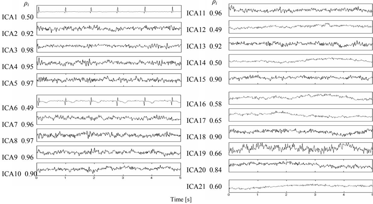
Figure 4: The independent components extracted from the MEG data measured with tone burst stimuli. The number to the left of each trace is the value of  $\rho_i$  measured with respect to the signal subspace (see text). Cardiac activity have been extracted (ICA1, ICA6), and found to have small values of  $\rho_i$  as expected. ICA14, 16 and 17 show small values of and thus were treated as noise; they may probably due to some drift in measurement system.
