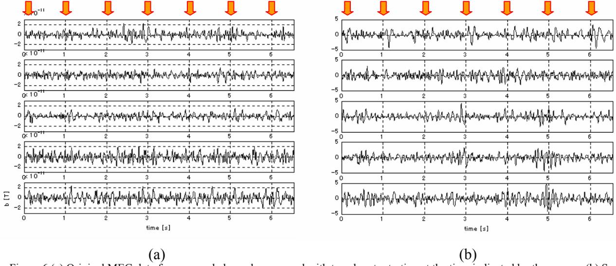
Figure.6 (a) Original MEG data from several channels measured with tone bursts starting at the time indicated by the arrows. (b) Some of the extracted independent components.
