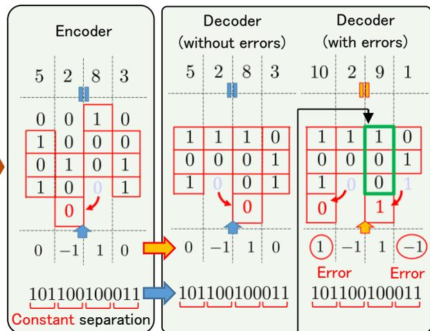
Most significant bits where bit assignments are true are guaranteed even when errors occur in the frame
