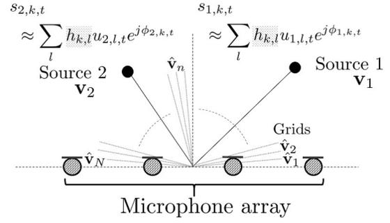
Fig. 1. Signal model for plane wave decomposition using linear array of microphones.
