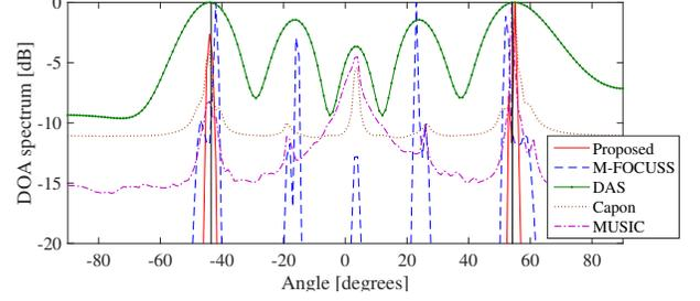
Fig. 2. Examples of DOA spectra for each method when the true angles were set to  $-43.5^\circ$  and  $54.2^\circ$ .
