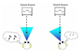
**figure 5.** Volume change according to the relative angle between head orientation and sound source
