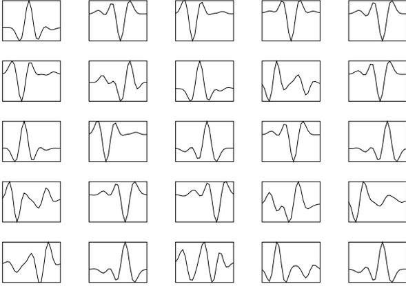
**Fig. 7.** B-ICA used for blind deconvolution. Plotted are the twenty-five rows of  $\tilde{\mathbf{B}}$  computed using B-ICA and the data in Fig. 6c.
