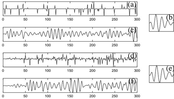
**Fig. 8.** B-ICA used for blind deconvolution. (a) A sparse spike train convolved with (b) the thirty-five point filter,  $\mathbf{h}$ , produces (c) the signal,  $\chi(t)$ . (e) The recovered filter,  $\hat{\mathbf{h}}_*$ , and (d) the independent component using B-ICA and the criteria in Eq. (14). (f) The convolution of (d) and (e).
