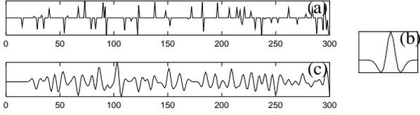
**Fig. 6.** B-ICA used for blind deconvolution. (a) A sparse spike train convolved with (b) the twenty-five point filter,  $\mathbf{h}$ , produces (c) the signal,  $\chi(t)$ . Given the data in (c), B-ICA finds the information,  $\tilde{\mathbf{B}}$ , presented in Fig. 7.
