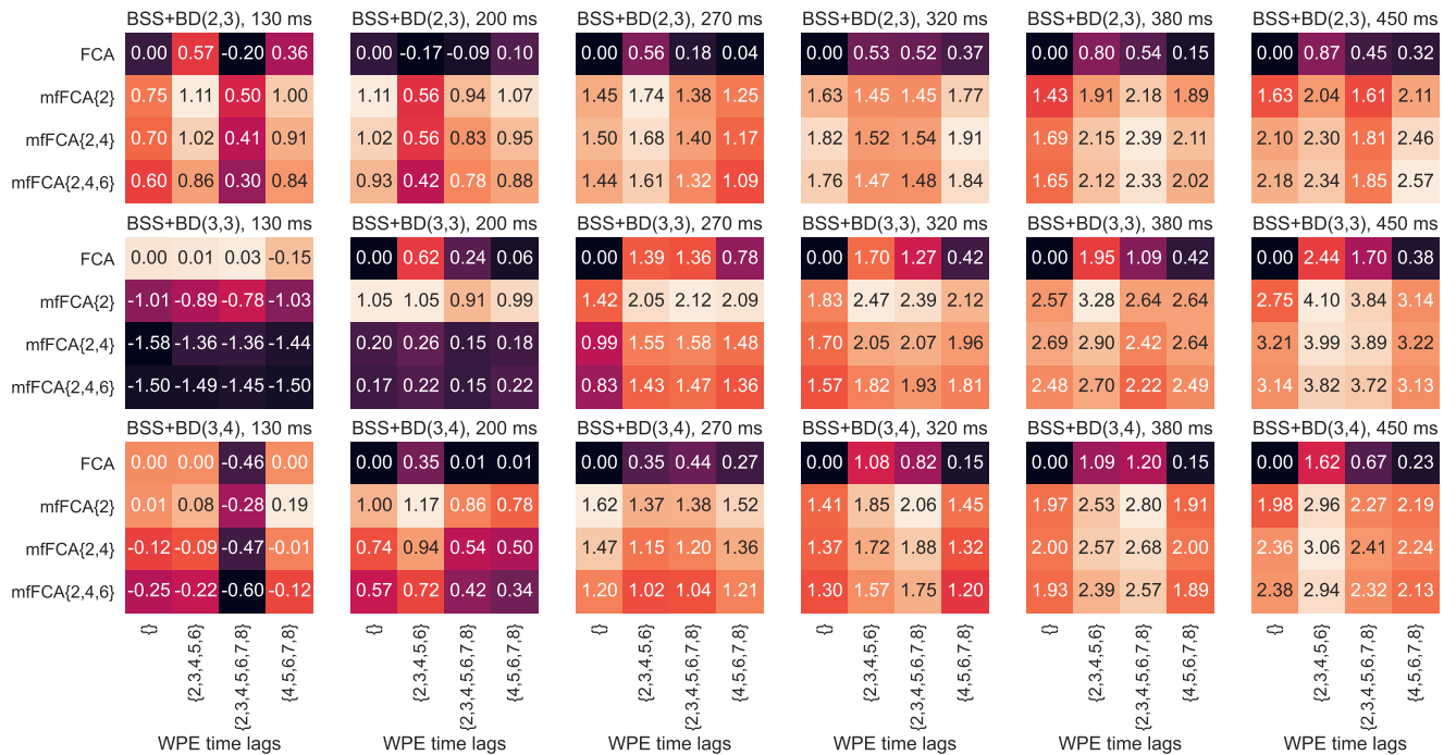
Fig. 7. BSS+BD performances when WPE was employed as preprocessing. The numbers in the colors represent the averaged SDR differences from the baseline, i.e., FCA without WPE. The three rows correspond to (M, N) combinations (2,3), (3,3), and (3,4). The columns correspond to reverberation times.
