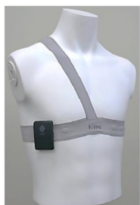
Appearance and electrode arrangement of wearable tensor electrocardiograph
